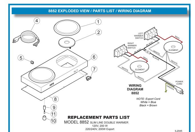
8852 Slim Line Double Warmer 8852 8852 UK 8852 EU Description Part No. Fig No PLATE COVER WARMER 2D-70090 1 2N-70091UL 2 ELEM WARMER FLAT 120V 100W 2N-70636UL 4 CORD & CAP A6-WL0412 A6-WL0140 A6-WL0141 5 2K-70215 STRAIN RELIEF STR 2K-70648 6 E5-WL0136 BODY, WARMER 7 SWITCH ON-OFF LITED 120V 2E-72946 2E-70247 8 PANEL BOTTOM E5-Z13605 9 FERRULE EYELET 2C-70316 10 BUMPERS RUBBER BLACK DD-70315 11 SCREW 8X1/2 PH PAN DRILL 2C-301522
